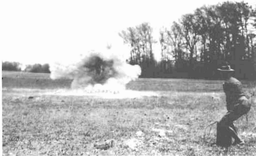
Test fire of a Livens Projector battery. The bombs are visible at the top of the picture. Note the bombs' tendency to tumble even at this early stage in the trajectory.
