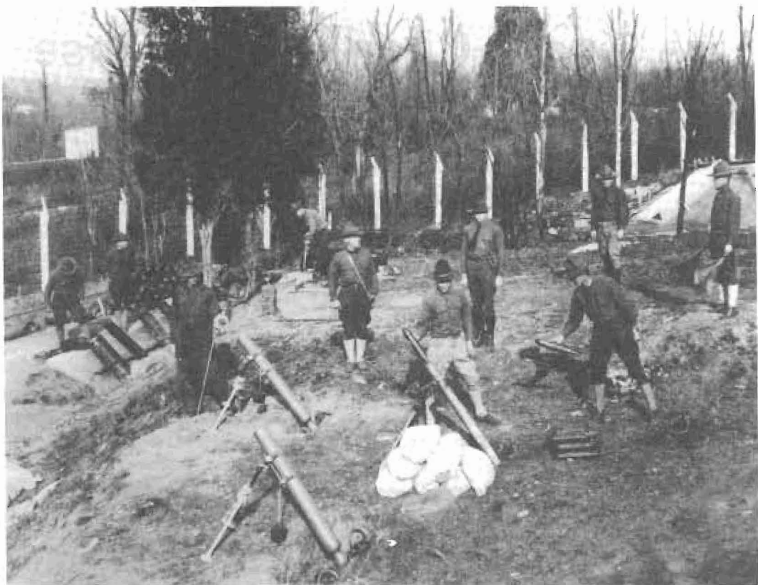
An inter-war target practice. The Livens Projectors and bombs are to the left. The weapons in the foreground are 3- and 4-inch Stokes Mortars, precursor of the 4.2-inch chemical mortar.
