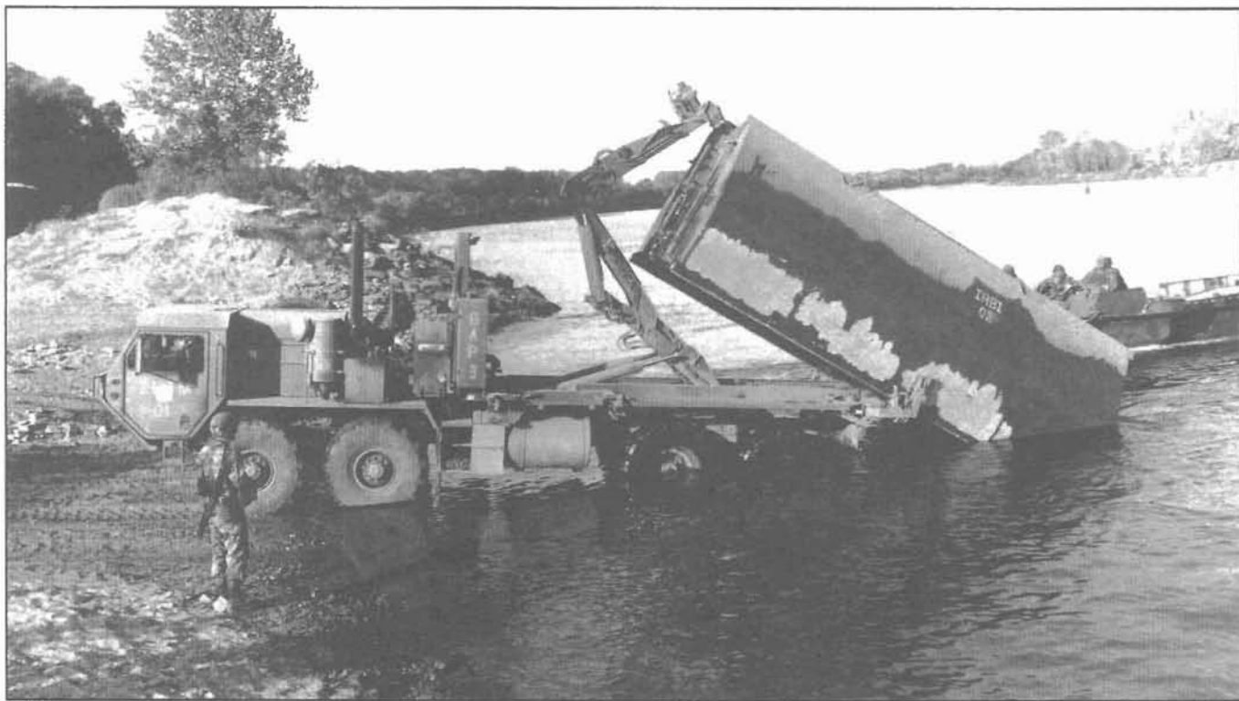
A HEMTT-based improved common bridge transporter from a corps multirole bridge company recovers a ribbon bridge bay.
