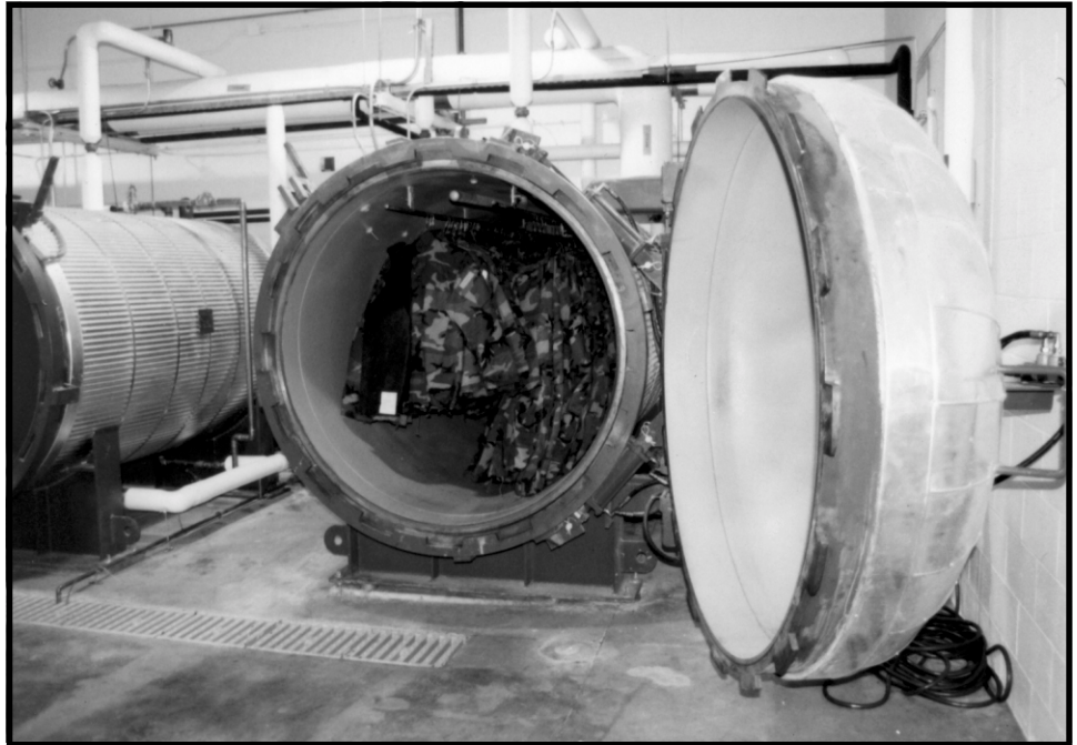
The chemical suits are put through an autoclave unit to ensure proper hygiene.
