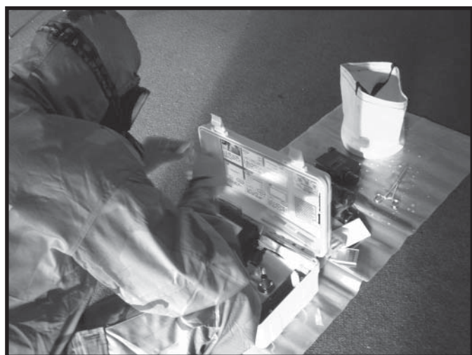
TE Soldier conducting presumptive identification of an unknown liquid
