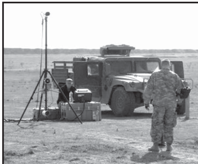
Soldier using the Sweep Monitoring System to calibrate an AN/PSS-14
