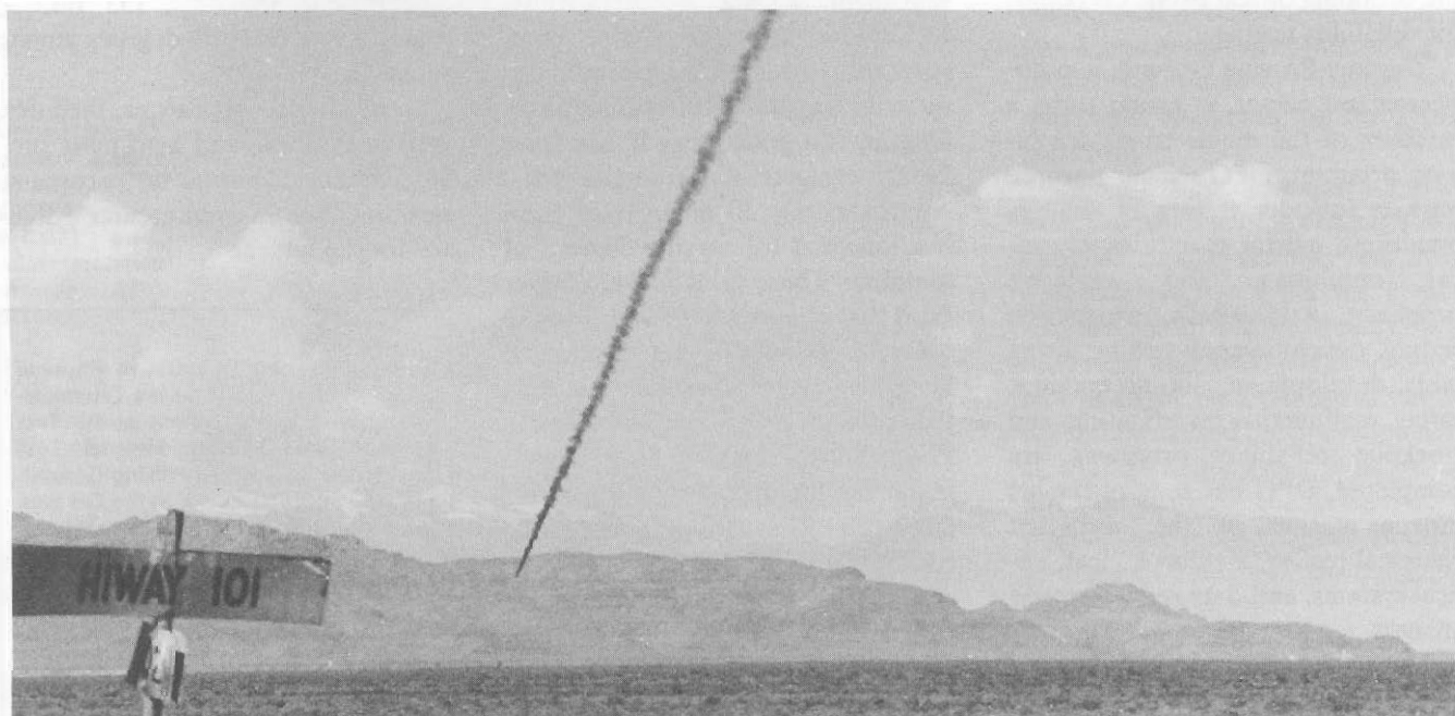
A simulant with red dye disseminates on Target S Grid at Dugway Proving Ground. Simulant was disseminated from a BIGEYE bomb.
