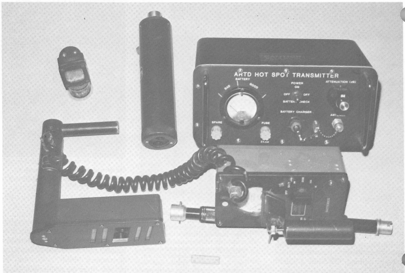
The Radiac Set Trainer (RST), a replica of the AN/PDR56 Alpha Radiac Detector, uses radio waves to simulate alpha radiation, giving the commander with a nuclear accident/response assistance mission the ability to train without the hazard of real alpha radiation.
