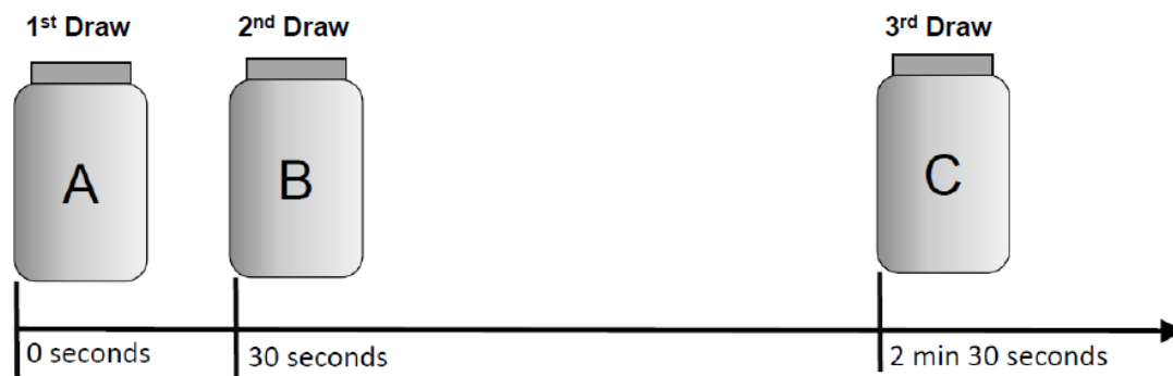
Figure 2: Timing of sample collection set after a water stagnation period of at least 8 hours using 250-milliter samples containers.
