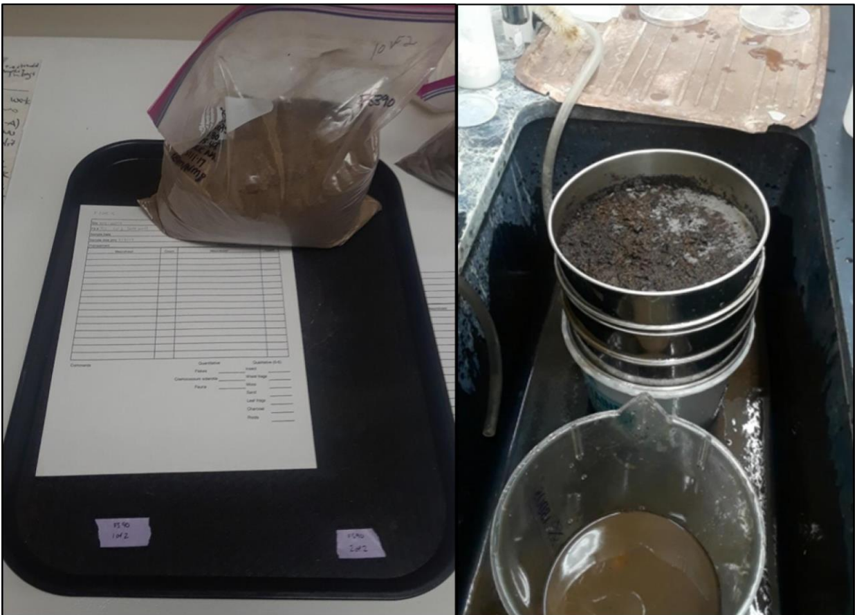
Figure 9.3. Bulk sample of feature matrix and wet-sieving system.
