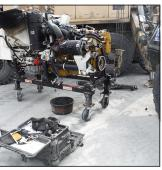
Drip pans must be placed under tactical vehicles. Winter temperatures can increase the rate of leaks – regularly monitor parked vehicles. Properly store all hazardous materials. Use dry methods to clean up spills ASAP and properly dispose of contaminated materials. Oily engine parts should not be exposed to weather, which could result in contaminated storm water runoff.
