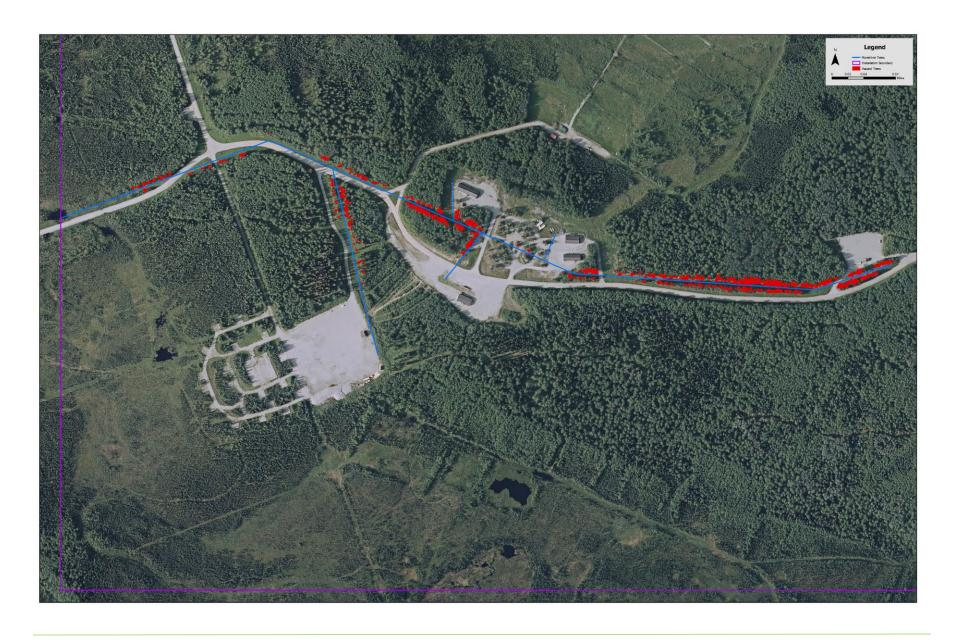
Vegetation Height was derived from LiDAR and used to identify hazard trees across the Yukon Training Area growing adjacent to power lines. Trees will be removed to mitigate fire risk from downed trees on powerlines.
