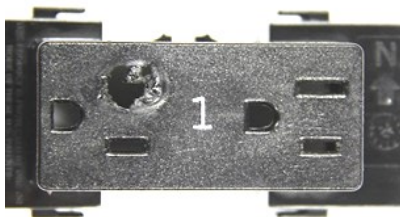
Receptacle damage from a loose connection.
