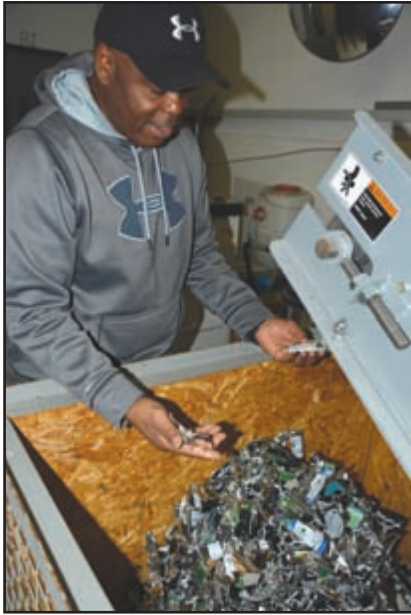
CDDF manager Curtis Burgess demonstrates how the hard drive shredder turns drives into scrap.
