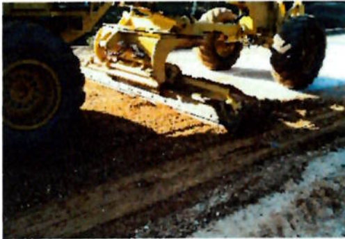
Proper moldboard forward tilt for blading.
