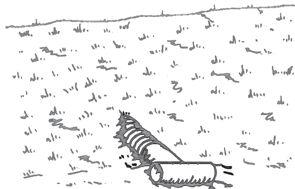
T-fitting on CMP Outlet
