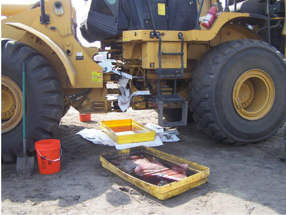
Down 966H CAT front end loader with a leaking hydraulic line
