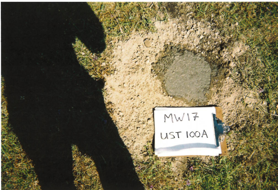
UST 100A: Well Abandonment – MW17
