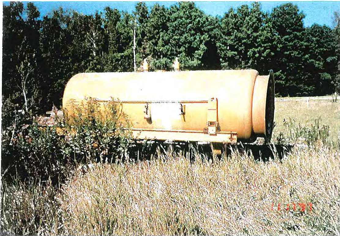
PHOTOGRAPH -13- ABOVE GROUND 1100 GALLON ALUMINUM STORAGE TANK
