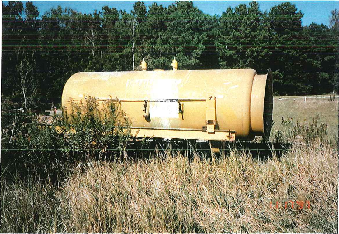
PHOTOGRAPH -13- ABOVE GROUND 1100 GALLON ALUMINUM STORAGE TANK
