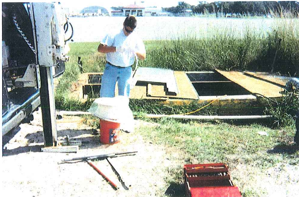
Pumphouse #6: Defuel Tank #92 Geoprobe sampling of HAA-PH6-6W-DF1. Groundwater 5.4' below ground surface. View to north, location southwest end of tank.
