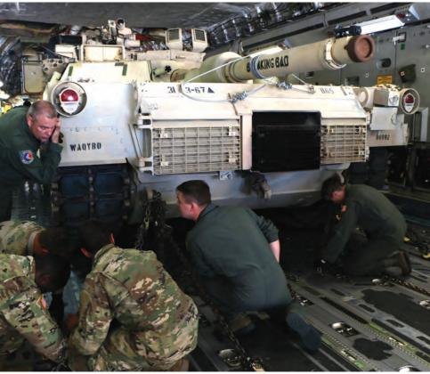
Soldiers with the 3-67th Armor, 2ABCT, 3rd ID, secure an M1A1-SA Abrams tank inside a C-17 Globemaster III, with the assistance of Airmen from the 15th Air Support Squadron, May 9, at Hunter Army Airfield.
