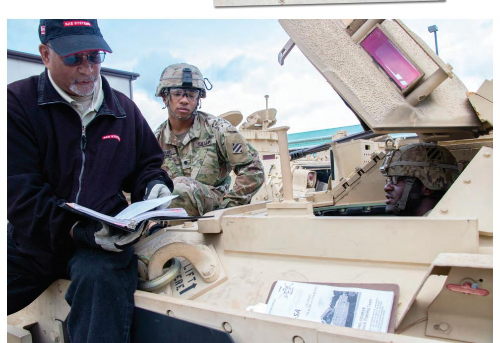
(From Left) A Department of Defense employee, Spc. Dorian Thomas and Pfc. Desmond Wilson of 6-8 Cav., 2ABCT, 3rd ID, conduct PMCS on the newly acquired M3 Cavalry Fighting Vehicle, Jan. 23, at Fort Stewart. PMCS ensures that a vehicle is fully mission capable and should not fail while in operation.
