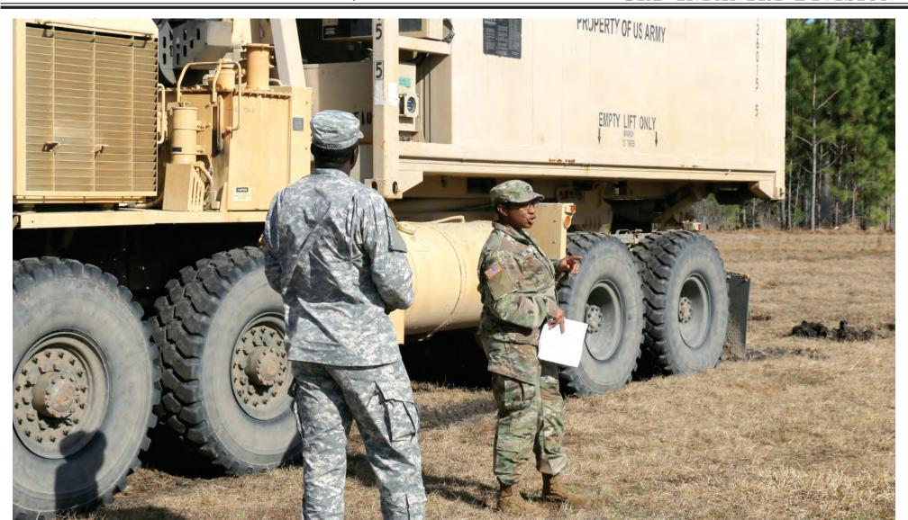
Sgt. Tomiko Jones and Sgt. Gerron Singleton, Culinary Specialists assigned to Co. I, 3-15 Inf., 2ABCT, 3rd ID, instruct a class on the Mobile Multi-temperature Refrigeration System, Jan. 23, at Fort Stewart. The MTRCS functions as a mobile refrigerator/freezer to store food in a field environment.
