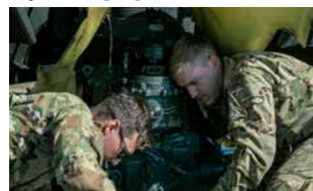
U.S. Army aircraft maintainers work on the combining transmission box of a CH-47 Chinook for a 160-hour phase maintenance inspection during a multinational training exercise. U.S. Army photo by SGT Jason Greaves.
