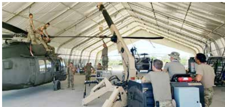
U.S. Soldiers conduct maintenance on a UH-60 Black Hawk helicopter using a self-propelled crane aircraft maintenance and positioning (SCAMP) II expeditionary crane. The SCAMP II is used to move major pieces of the helicopter. U.S. Army photo by SFC Melanie McCracken.
