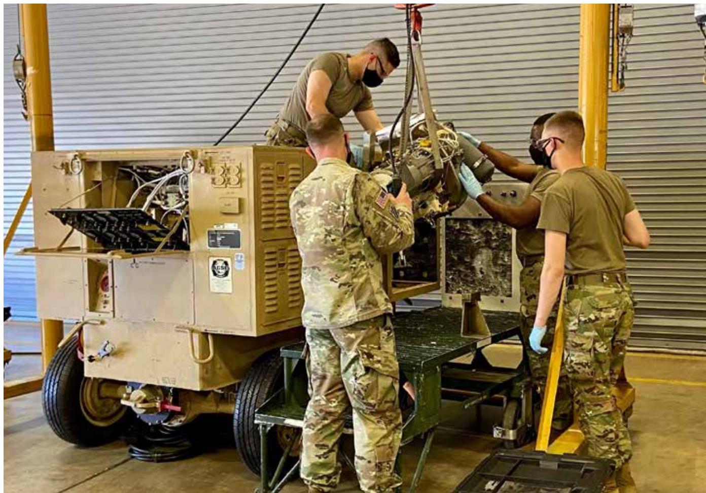
U.S. Army Soldiers hoist the engine of an Aviation Ground Power Unit off of a maintenance stand at Fort Eustis, Virginia. U.S. Army photo by SSG George Prince.
