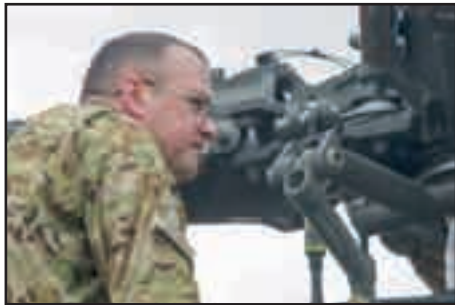
PHOTO BY SGT. WILLIAM BEGLEY CW2 Eric Leon, maintenance test pilot, inspects the main hub on an AH-64 Apache.
