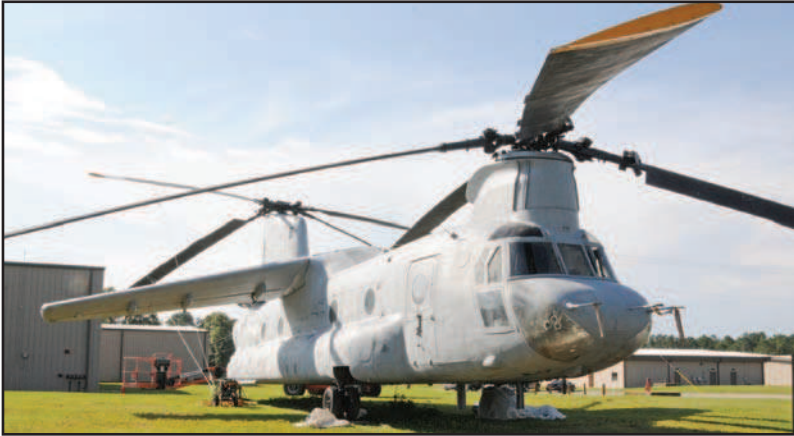
The BV-347 that sits on the west lawn of the U.S. Army Aviation Museum was a technology demonstrator that was retrofitted with improvements from a CH-47A model.
