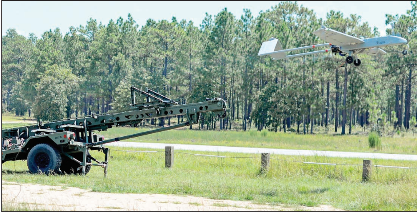
An RQ-7BV2 Shadow UAS propels off its launcher at about 80 mph at an airfield near Fort Bragg Aug. 18.
