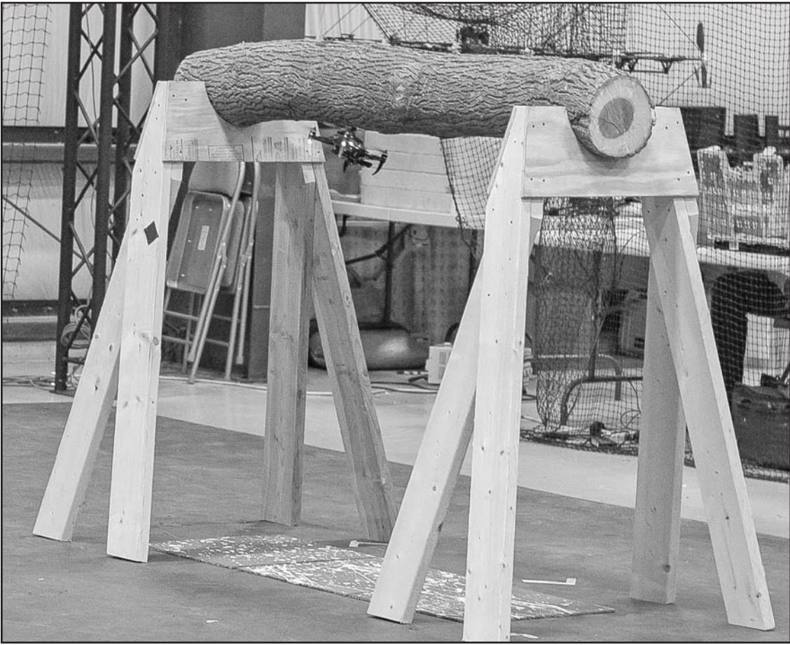
University of Pennsylvania researchers demonstrate a successful perching technique where an autonomous quadcopter attaches itself to a log.
