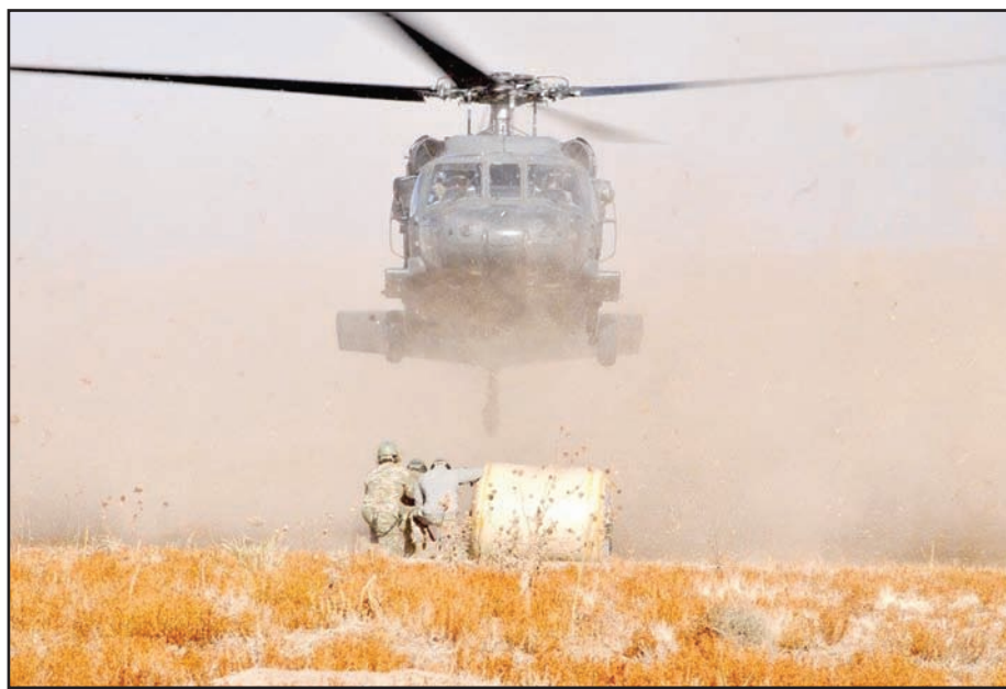
A UH-60 Black Hawk assigned to the 4th CAB approaches awaiting 10th SFG Soldiers preparing to hook up a 500-gallon water blivet during sling load training at a Fort Carson, Colo., training area.
