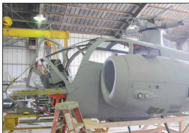
**The XH-51 Compound helicopter was an evolutionary aircraft that utilized a four-bladed, rigid-rotor system, along with stub wings with an auxiliary 2,900-poundforce J60-2 engine mounted on one side for added thrust. The one-of-a-kind aircraft sits in the U.S. Army Aviation Museum's collection and is undergoing restoration.**
