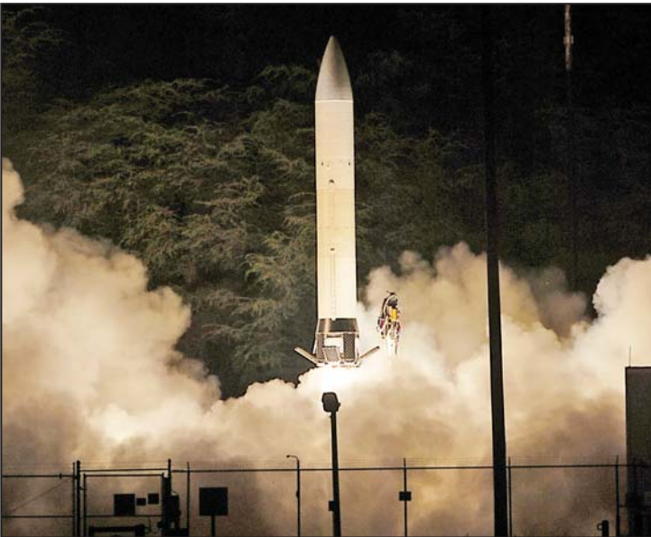
The U.S. Army Space and Missile Defense Command/Army Forces Strategic Command conducts the first flight of the Advanced Hypersonic Weapon concept Nov. 18. The AHW is a first-of-its-kind glide vehicle, designed to fly within the Earth's atmosphere at hypersonic speed and long range. It was launched from the Pacific Missile Range Facility, Kauai, Hawaii, to the Reagan Test Site, U.S. Army Kwajalein Atoll, Marshall Islands.
