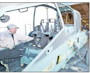
A Boeing shipping and receiving employee rolls the fuselage of the first AH-64D Anache Block III helicopter on to the receiving dock as it arrives at the Mesa, Ariz., facility Jan. 28.
