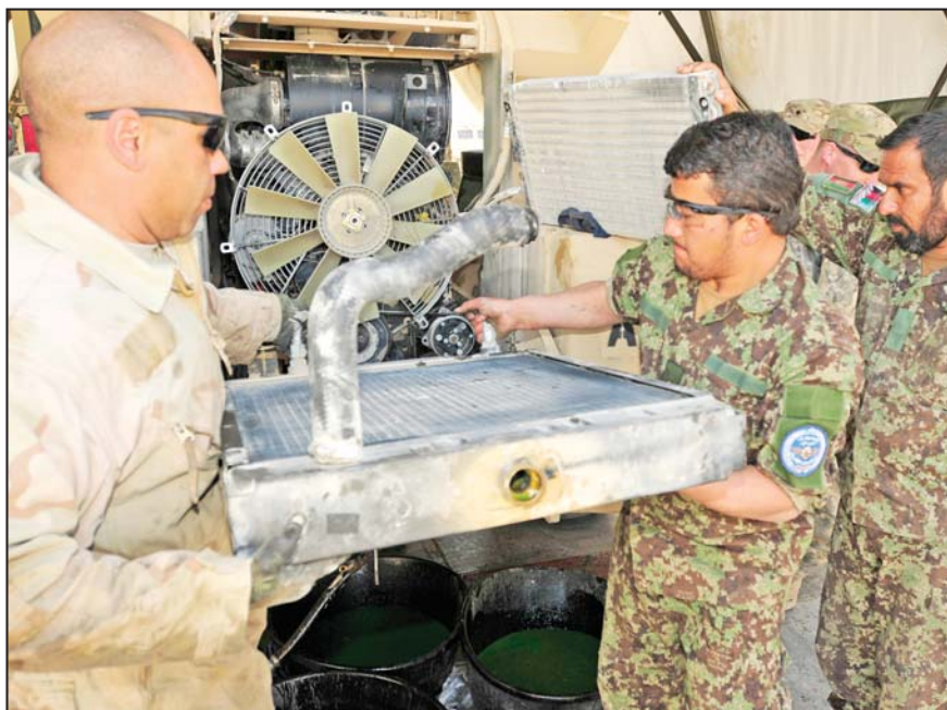
Spc. Sergio Ortiz, a wheeled vehicle mechanic assigned to Headquarters Support Company, 209th ASB, 25th CAB, and Sgt. Mohammad Rajab, a mechanic with 205th Corps, Afghan National Army, use teamwork to remove the radiator of a forklift during a vehicle maintenance training session at the motor pool on Kandahar Airfield, Afghanistan, March 8.
