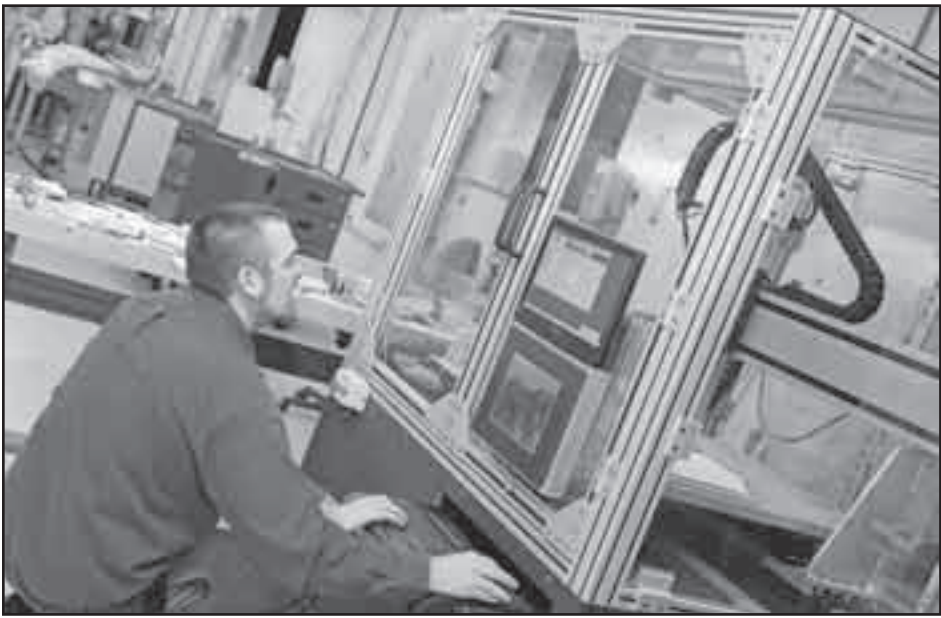
Zunino displays a modular tool that can be added onto the Multi-Axis Modular Manufacturing Platform for additive manufacturing. Different tools allow the machine to perform different manufacturing techniques.
