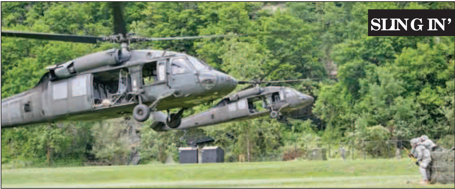
PHOTO BY SGT. 1ST CLASS JEREMY BUNKLEY Trainees in West Point Air Assault Course 15-2 participate in the hands-on portion of the sling load operations phase June 6. During this phase, students learn how to rig equipment onto rotary aircraft with a sling, an operation that generally requires the loading Soldier to hook a tether to the underbelly of a helicopter hovering just a few feet above the ground. The Air Assault mobile training course is taught by instructors from the Sabalauski Air Assault School, Fort Campbell, Ky., and runs in four iterations throughout the summer.
