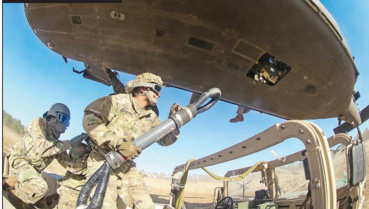
Soldiers with 127th Engineer Battalion, 1st Brigade Combat Team prepare to connect a high-density load to the belly of an UH-60 Black Hawk helicopter assigned to 82nd Combat Aviation, 82nd Airborne Division during a sling load training event at Latham pick-up zone on Fort Bragg, N.C., Dec. 7.
