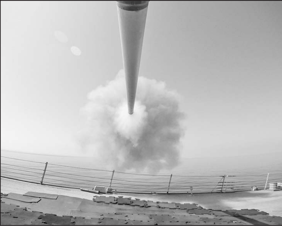
NAVY VIDEO The Office of Naval Research electromagnetic railgun industry prototype launcher is being evaluated at the Naval Surface Warfare Center, Dahlgren Division. The railgun is a long-range weapon that launches projectiles using electricity instead of chemical propellants.
