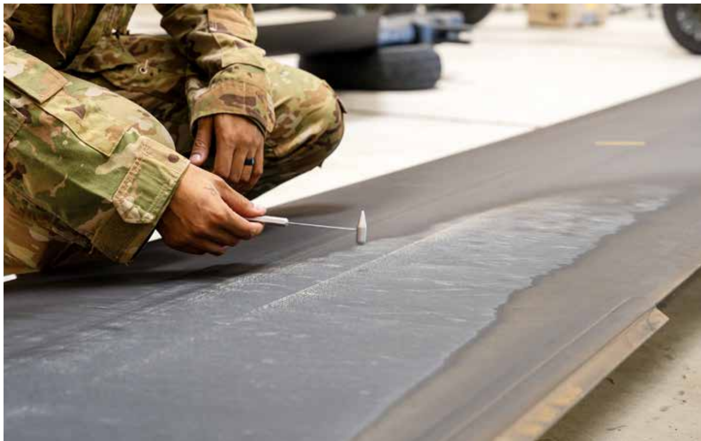
4th CAB Soldier performing a tap test after the microburst. Photo provided by the 4th CAB.
