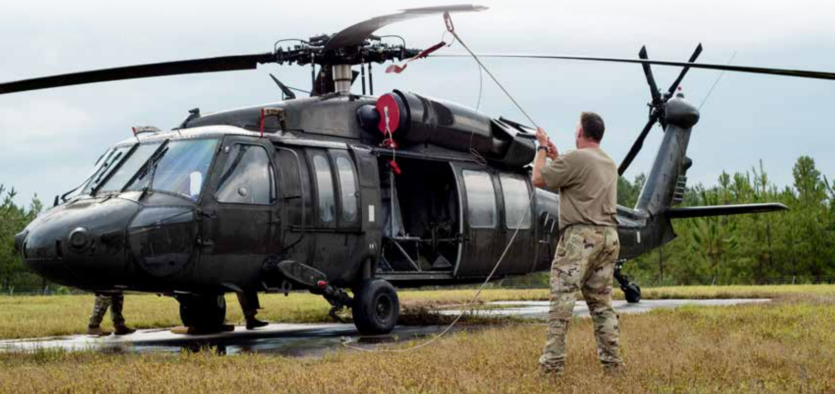
A flight crew member ties down the rotor blades of a UH-60 Black Hawk prior to inclement weather. Mississippi National Guard photo by SGT Shawn Keeton.
