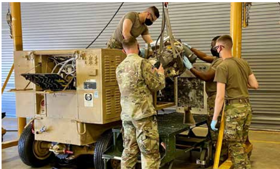
Soldiers hoist the engine of an Aviation Ground Power Unit off a maintenance stand at Fort Eustis, Virginia. U.S. Army photo by SSG George Prince.
