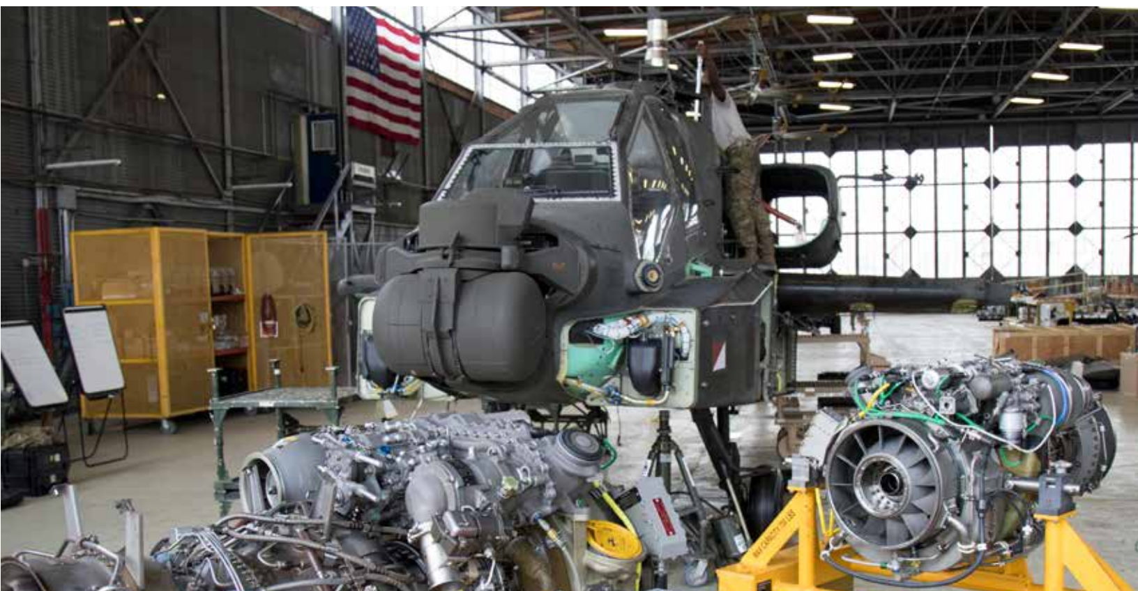
The engines of an AH-64 Apache helicopter await to be hoisted and connected to the helicopter while a Soldier inspects the inside on March 22, 2017. This is a part of phase maintenance conducted by 603rd Aviation Support Battalion, which supports the 3rd Combat Aviation Brigade by performing maintenance, providing maintenance support, and performing intermediate-level maintenance on components, subsystems, and airframes. U.S. Army photo by SGT Kellen Stuart, 3rd CAB Public Affairs
