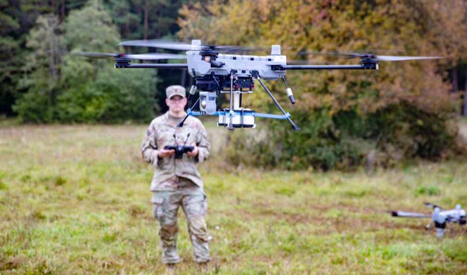
A U.S. Soldier from the 101st Airborne Division monitors a PDW C-100 drone in flight, outfitted with the Widowmaker munition dropper, during exercises in Germany. U.S. Army photo by SPC Adrian Greenwood.
