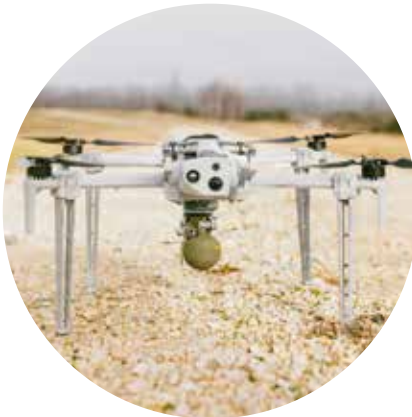
A Skydio drone equipped with a U.S. Army Combat Capabilities Development Command–designed dropper system sits staged for a demonstration during a Live Drop 5.0 exercise at Grafenwoehr Training Area, Germany. U.S. Army photo by SFC Arturo Guzman.
