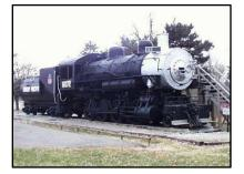
Locomotive #6072 symbolizes the importance of the railroads in the development of the West. The railroad arrived at Fort Riley in the fall of 1866. The Union Pacific Railroad donated this 110 ton locomotive to Fort Riley in February 1958. The engine was built as a coal steam engine in 1908 and converted to an oil-burner in 1941. The engine was used on mid-western rail lines for nearly a half century before coming to Fort Riley.
