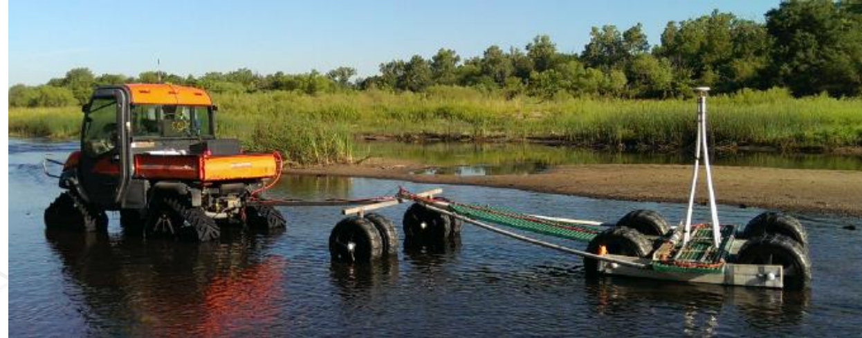
EM61 towed array water survey
