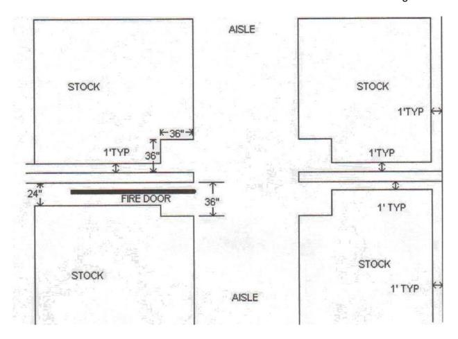
NOTE: STACK CLEARANCE SHOWN ABOVE ARE NOT REQUIRED WHERE FIRE DOORS ARE PROTECTED BY PERMANENTLY INSTALLED FIRE DOOR GUARDS WHICH PREVENT STOCK INTERFERING WITH FREE OPERATION OF FIRE DOORS.
