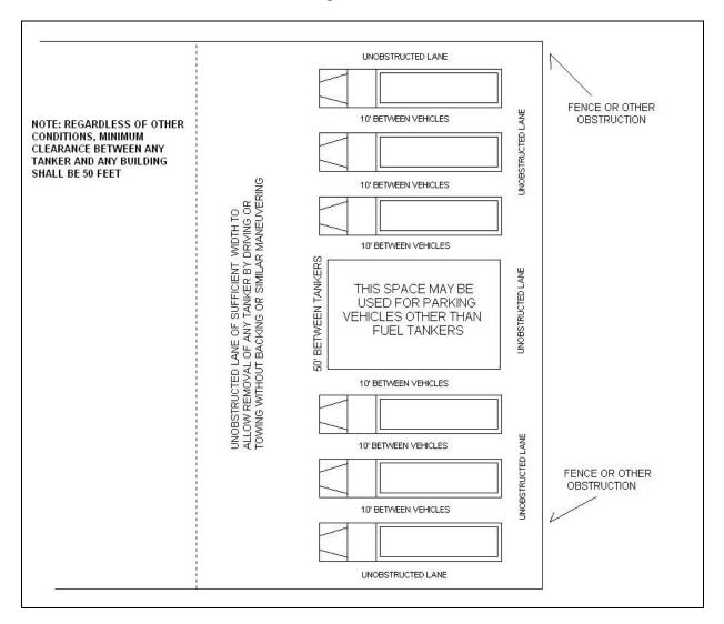
Figure 11-1. Parking For Fuel Tank Trucks
