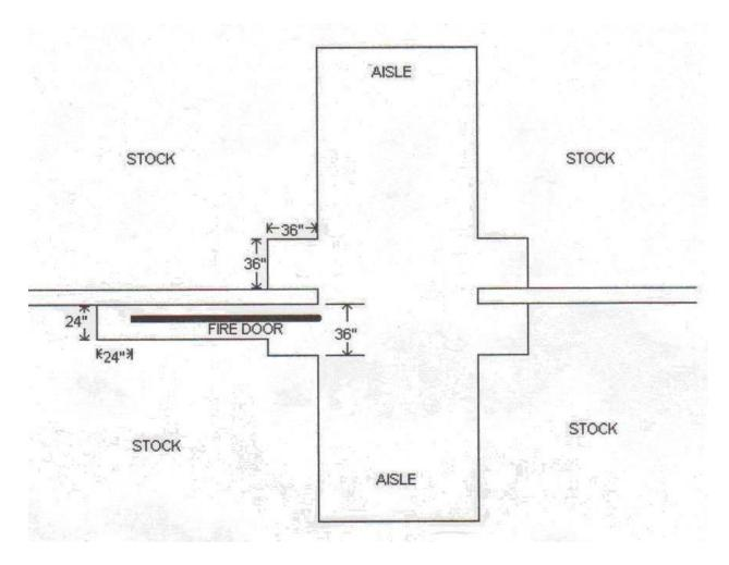
NOTE: STACK CLEARANCES SHOWN ABOVE ARE NOT REQUIRED WHERE FIRE DOORS ARE PROTECTED BY PERMANENTLY INSTALLED FIRE DOOR GUARDS WHICH WILL PREVENT STOCK INTERFERING WITH FREE OPERATION OF FIRE DOORS.
