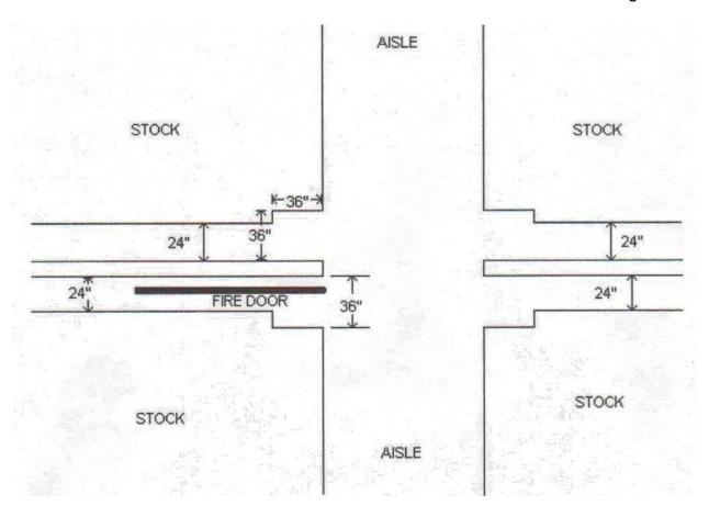
Figure B-4 – Stack clearance at substandard fire walls.
