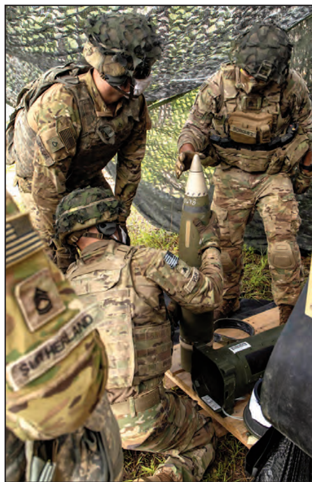
Sgt. 1st Class Manuel A. Borquez, master gunner for 5th Battalion, 25th Field Artillery Regiment, 3rd Brigade Combat Team, 10th Mountain Division, inspects an M982A1 Excalibur round prior to loading it into an M777 howitzer for a live fire training event June 27 at firing point 700.
