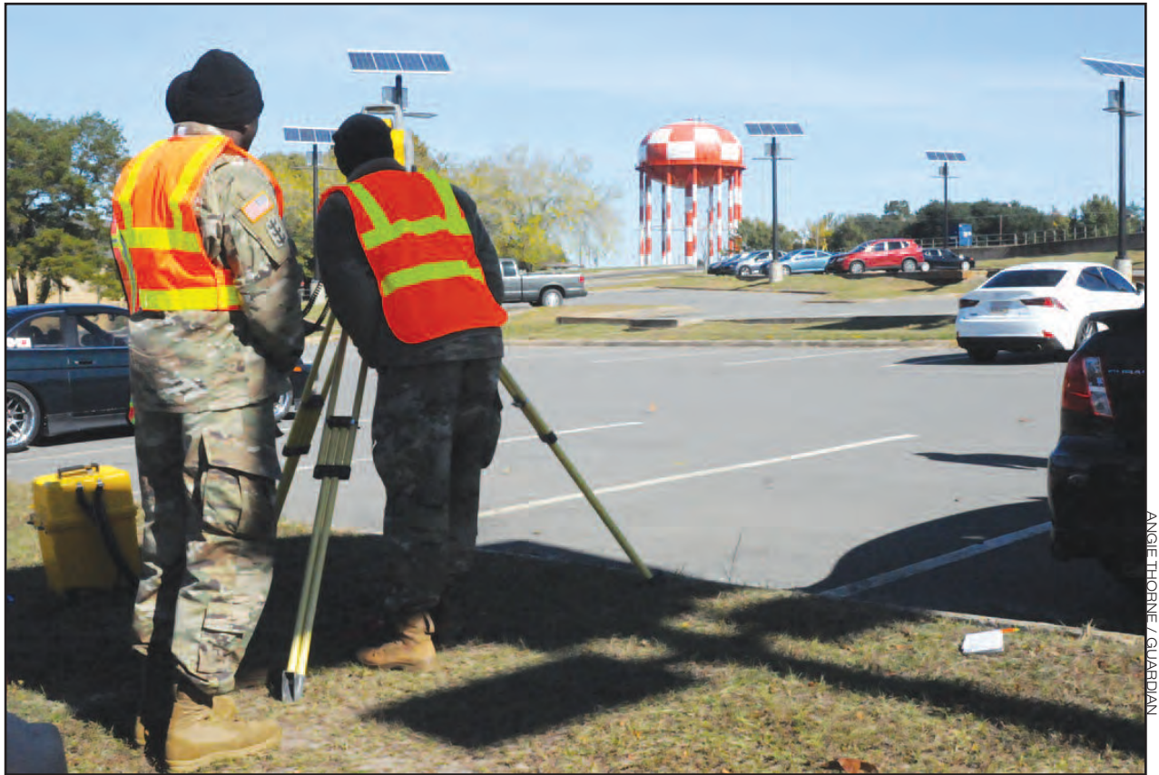
A 46th Engineer Battalion field survey team measures the GPS and elevation coordinates of a Fort Polk water tower Nov. 12.
