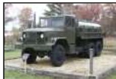
Designed in the 1950s, this truck was used to haul and discharge gasoline and jet fuel. Each of its 600-gallon stainless steel tanks used a delivery pump and metering system. The delivery pump, located in the compartment at the rear of the body, also was used to
