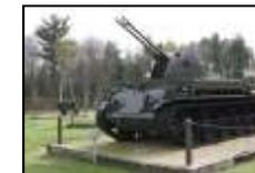
Manufactured by Cadillac in 1951, the M42A1 deployed with armored divisions as a means of providing mobile anti-aircraft weapons. Because of its rapid rate of fire, it also proved valuable as an infantry support weapon against ground targets. **Crew:** 6 (commander, gunner, sight-setter, two loaders, driver). **Armament:** 2 - 40 mm guns.
