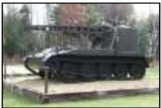
The M578 originally was developed as a heavy-lifting crane for barrel replacements of self-propelled guns in heavy-artillery battalions and was used as such in the 1970s. Today, the M578 functions more as a wrecker
