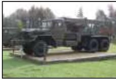
The M819 was used for wrecker, hauling, and salvage operations. Its hydraulically-powered, engine-driven crane could extend 11.5 to 26 feet, rotate 270 degrees, and elevate 45 degrees. It is also equipped with a fifth wheel for hauling semitrailers and a front winch to free the vehicle when it becomes mired. **Crew:** 2. **Top Speed:** 45 mph.
