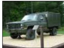
The M1031 is part of the Commercial Utility Cargo Vehicle series. It has a chassis and cab combination, designed for the mounting of special bodies that might be required. The trucks are powered by a V-8 diesel
