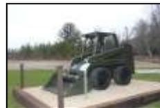
Often referred to as a skid loader or skid-steer loader, the Bobcat is a small, rigid framed, engine-powered machine with lift arms used to attach a wide variety of labor-saving tools or attachments. The main use is for excavating and earth-moving work. Skid-steer loaders are capable of zero-radius, "pirouette" turning, which makes them extremely maneuverable and valuable for applications that require a compact, agile loader.
