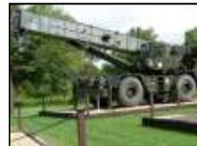
The RTCC is a wheel-mounted crane that serves as a container handler. It is a non-developmental item that is a military-unique integration of commercial components. More than 300 RTCCs were procured by the U.S. Army Tank-Automotive and Armaments Command from 1987 through the mid-2000s. The 40-ton RTCC has a hydraulically operated, full 360-degree revolving, telescoping boom designed to support 20- and 40-foot containers, using spreader bars, during inter-
