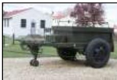
The M332 trailer is used to transport ammunition in tactical situations. **Artillery Round Carrying Capacity (number):** 8-inch (12), 155 mm (24), 105 mm (50). **Maximum Towed Speed:** highway, 50 mph; cross country, 25 mph. **Payload:** 3,000 lbs.
