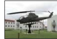
This single-engine attack helicopter's primary use was to destroy armored vehicles. It is equipped with Hydra 70 multipurpose submachine rockets and 20 mm cannons, which are effective against other targets. **Crew:** 2. **Top Speed:** 129 knots. **Maximum Endurance:** 4 hours. **Rotor Diameter:** 44 feet. **Armament:** TOW missiles, 2.75-inch rockets, 20 mm cannon.
