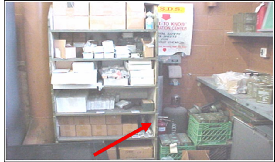
Flammable gas cylinder stored with corrosive/reactive material
