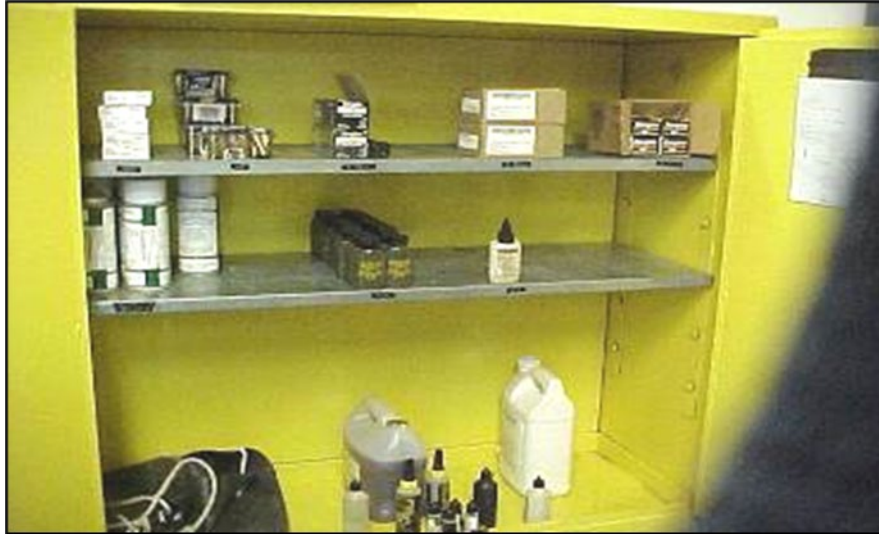
Corrosives and flammables stored together
