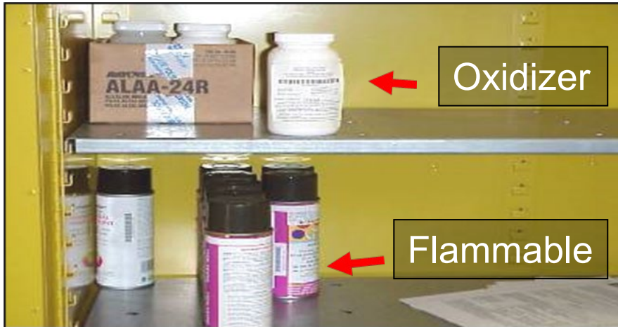
Oxidizer stored with flammable paints
