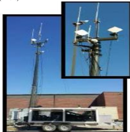
HITS RBS Trailer with RTKI Antenna Kit: GPS/Telemetry Antenna Installed
