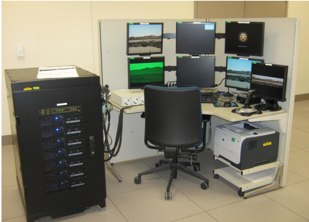
Instructor/Operator Station (IOS) with a Crew Station in the background
