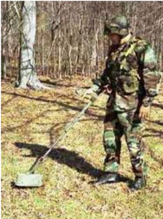
Sweep Monitoring System showing optical tracking target mounted on tracking head of mine detector
