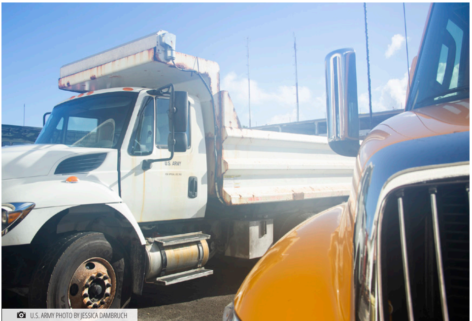
I give it four months: The front fender of a shiny, yellow work vehicle, right, is headed for the rusty fate of it’s neighbor in the yards at Kwajalein Automotive. Corrosion control is a regular part of island vehicle maintenance. Operators can assist by rinsing their cars and trucks at the end of the day.
