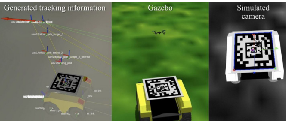
In this U.S. Army photo, researchers show the data and coordinate frame visualization during landing, Middle: Gazebo simulation view, Right: Simulated camera view with marker detection overlaid.
