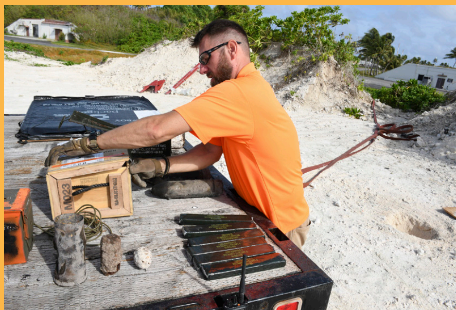
RGN EOD Tech Matthew Hess readies plastic explosives and unexploded ordnance for demolition at a Kwajalein blast site March 12. Among the tools for the day's work are a retaining barrier, bars of C-4 and detonating cord.
