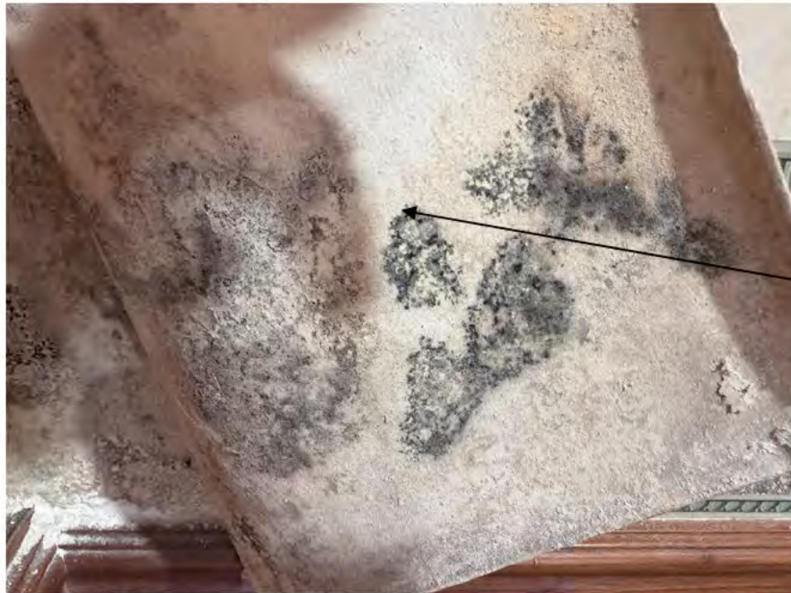
Photo 23: Mold growth observed on the backside of wallpaper in Dining Room 130 (Sample #M3).
